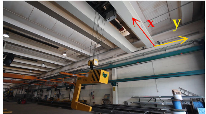
Fig. 3. The real bridge crane used for the tests. The X and Y axes are super imposed.
