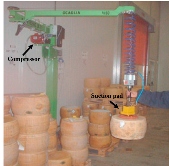
Fig. 2. Example of operating condition of the device in food industry. Notice that the manipulator in this picture is equipped with a suction-pad: vacuum is done inside the pad by a pneumatic compressor, the load is attached to the handling device and can be moved.
