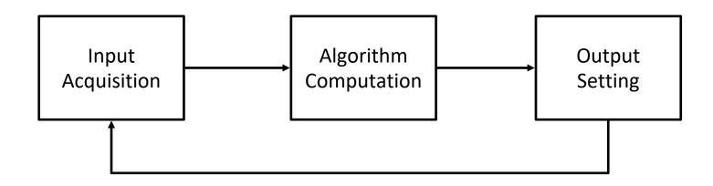
N.B.: Usually the relaunch time of the execution cycle is fixed. However, sometimes with some PLCs (such as Siemens') if you don't define a function block with a fixed sampling time, the code is executed in an "infinite loop" (in a main function with a "while true" loop). In that case is not possible to know the relaunch time.
