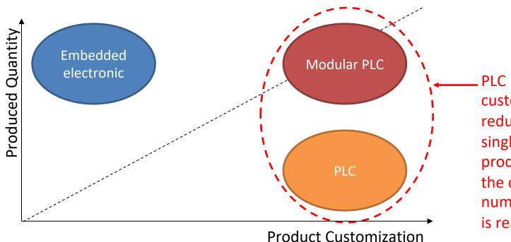
PLC is useful to develop customized systems in reduced number (or for a single-product, such as production lines), when the complexity and the number of I/O interfaces is really high
