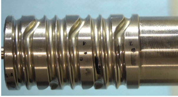
Fig. 8. The screw thread after the tests without lubricant. It is possible to notice the lucid areas where the balls passed, due to high contact pressures.
