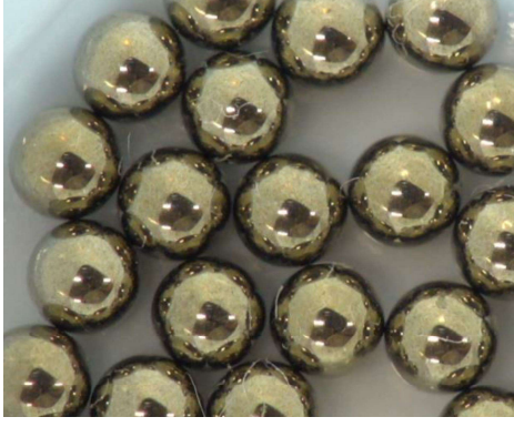
Fig. 7. Balls from one of the circuits after the tests without lubricant. They appear like hammered and opaque.
